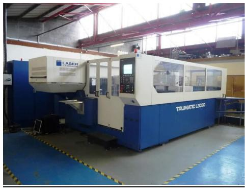
TRUMPF MAKE LASER MACHINE L3030 / 4 KW
